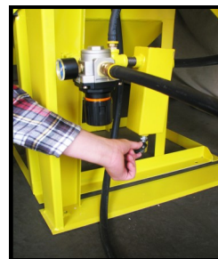
High flow air regulator with pressure booster and moisture separator
